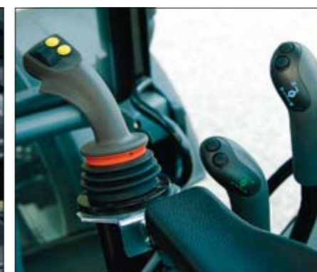
Danfoss – Profi joysticky s elektronickou reguláciou prietoku
